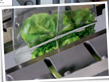
Above: An ultrasonic module incorporated into a horizontal form-fill-seal pouch line
