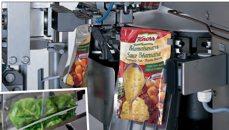
Above: An ultrasonic module incorporated into a horizontal form-fill-seal pouch line
